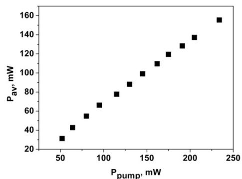
Figure 5: Dependence of pulse duration and average power from pump power after WDM.
