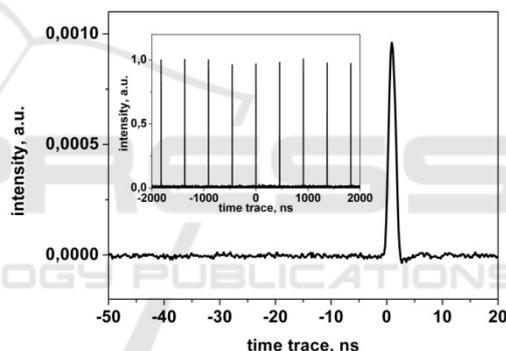
Figure 8: Time trace of the pulses in the PM scheme.
