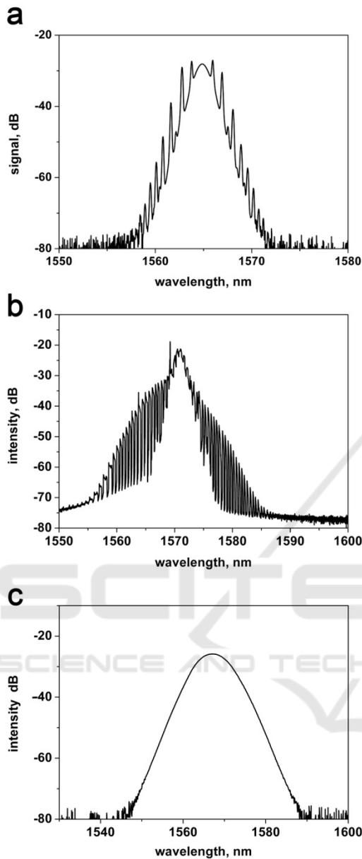
Figure 3: Spectrum of the pulses in all-anomalous dispersion non-PM scheme. a – solitons regime; b – regime of cooperative solitons and nanosecond pulse propagation; c – regime of nanosecond pulse propagation.
