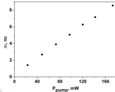
Figure 11: Dependence of pulse duration on pump power.
