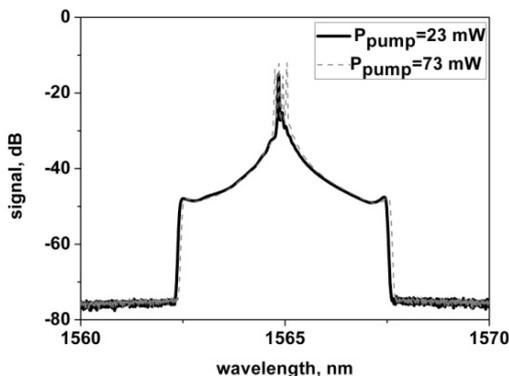
Figure 10: Measured spectrum of the pulses oscillating in all-normal dispersion scheme.
