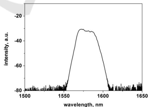
Figure 9: Measured spectrum of the pulses oscillating in the PM scheme.
