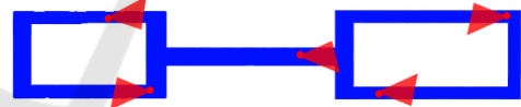
Figure 8: Configuration of cameras obtained by optimizing the cell coverage quality metric proposed by Janoos et al. 2007 for each cluster.(Janoos et al., 2007).
