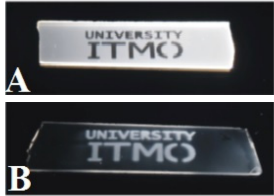
Figure 10: Negative and positive luminescent images in PTR glass plates irradiated through the mask by the UV nanosecond laser radiation with (A) and without (B) the preliminary irradiation by the UV mercury lamp.
