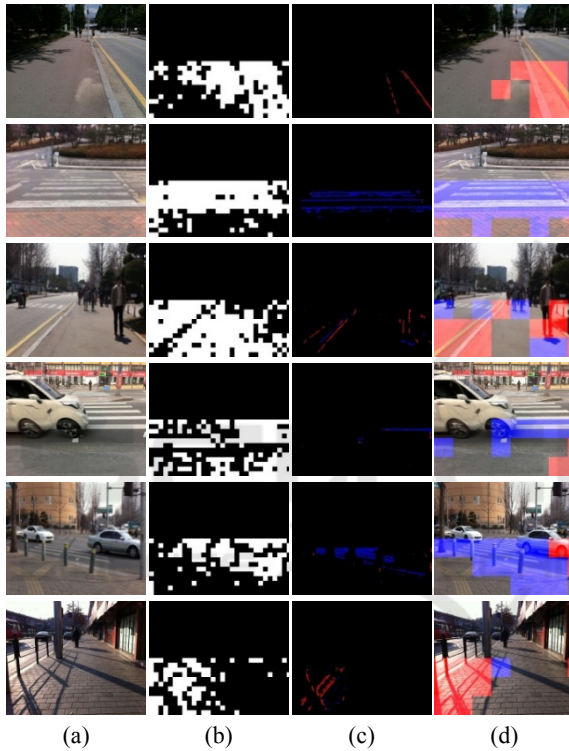
Figure 6: Context recognition results. (a) Input image, (b) boundary extraction results, (c) classification results, (d) final results after post-processing.
