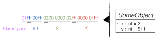
Figure 8: Data transformation for entity with two integer variables. Header contains a numeric namespace and a numeric identifier for SomeObject. Attribute values will be added after header in alphabetic order.
