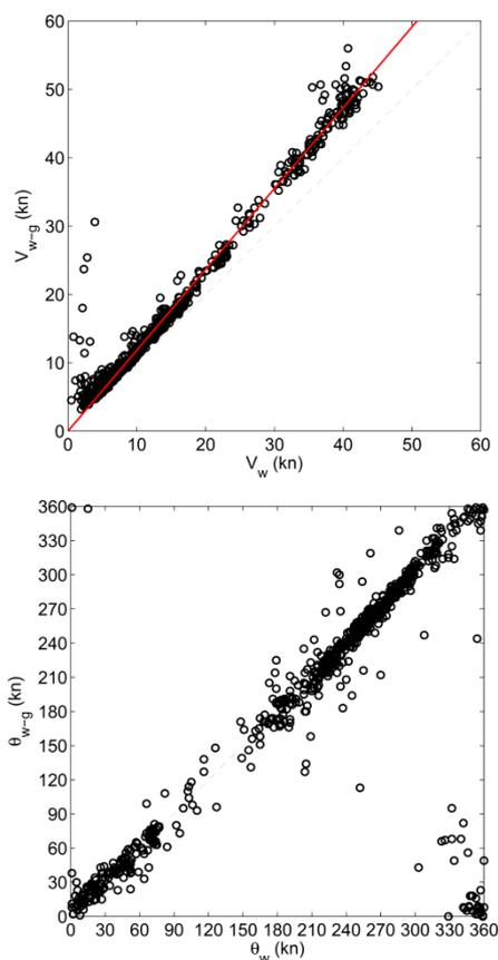
Figure 11: Upper panel: scatter plot between the averaged true wind speed and the true wind gust; the red line represents the functional relationship, as obtained by applying a linear regression to the measured data. Lower panel: scatter plot between the averaged true wind direction and the true wind gust direction.
