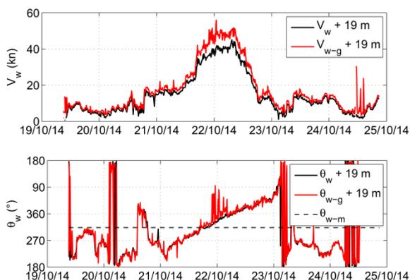
Figure 10: Upper panel: time series of the true wind speed averaged over 10 minutes (black line) and of the true wind gust (red line). Lower panel: time series of the true wind direction averaged over 10 minutes (black line) and of the true wind gust direction (red line); note: the dotted black line refers to the mean direction of the true wind ( $\theta_{w-m}$  during the event is  $313.6^\circ$ ).
