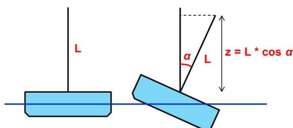
Figure 13: Sketch of the measurement height  $z$  as a function of the heeling angle  $\alpha$ .
