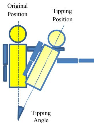
Figure 2: Schematic of maximum reach to right on frontal plane from original position to tipping position. Tipping angle is measured with reference to spine between the 2 positions.
