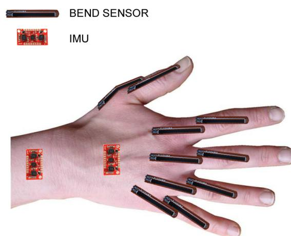
Figure 2: Sensors placings: ten flex sensors on-top of the MCP and PIP joints, one 6DoF IMU on the dorsal aspect of the hand, and one 6DoF IMU on the forearm. The supporting glove is not showed here for clarity reasons.
