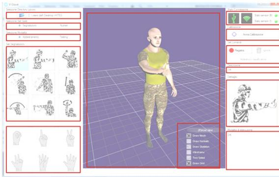
Figure 6: The graphical user-friendly pc-interface for training and testing purposes. On the right column the recognized gesture, on the middle column the animation of the selected gesture via human avatar.
