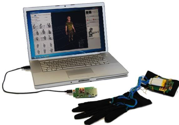
Figure 1: The “extended” sensory glove, the electronic circuitry (both the source and the receiving one), the virtual representation on a personal computer.
