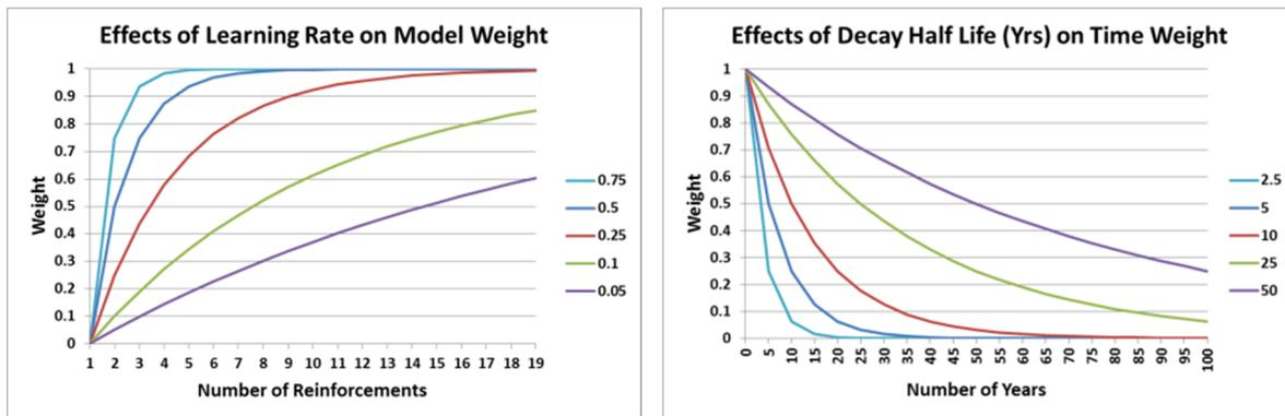
Figure 2: Left: Effects of Reinforcement Factor (Learning Rate) on Weight; Right: Effects of decay half-life on time (Forgetting Factor) weight.
