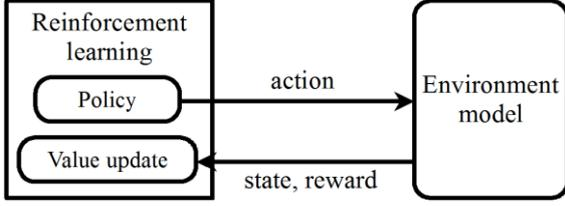
Figure 1: A reinforcement learning system (Sutton, et al., 1998).
