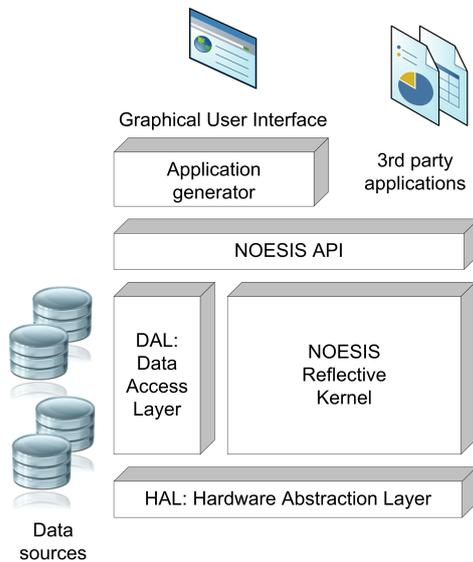
Figure 1: The NOESIS system architecture.
