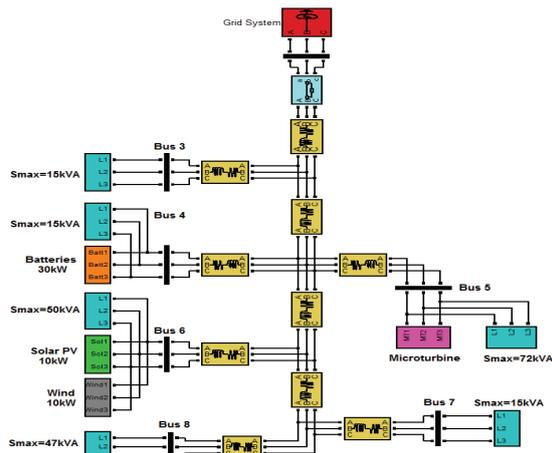
Figure 5: Benchmark LV microgrid networks using neural controllers.
