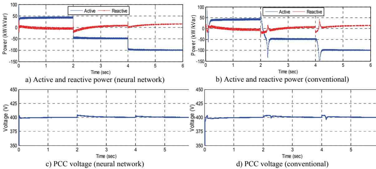
Figure 2: Performance of PV-inverter DER using conventional and neural network controllers ( $T_s=1ms$ ).
