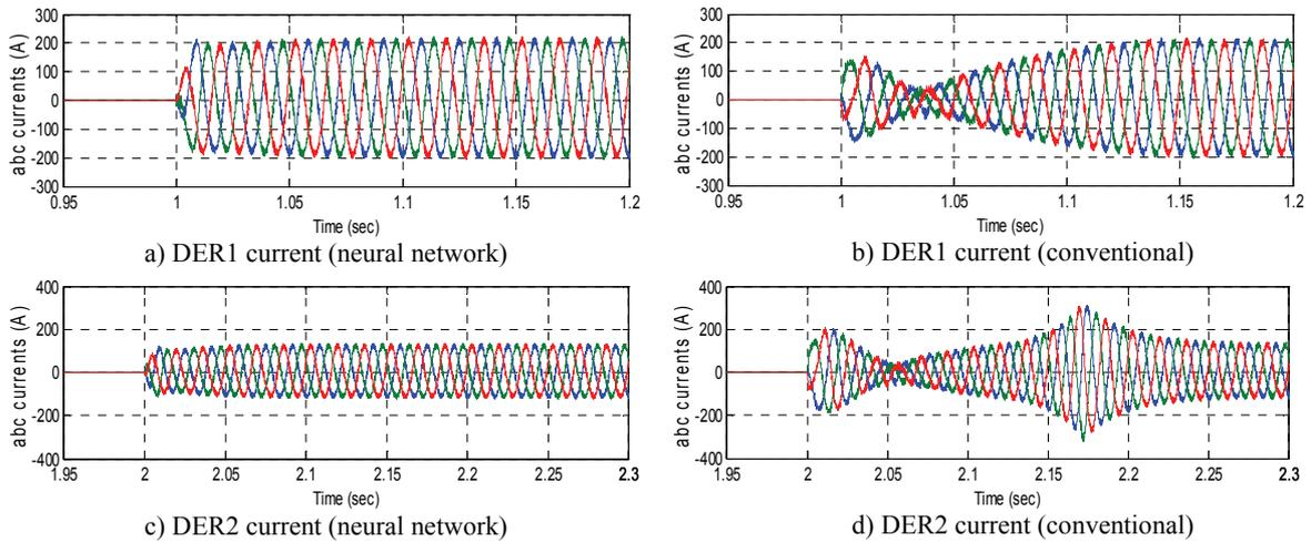
Figure 6: Three-phase currents when connecting DERs to the grid without synchronization control.
