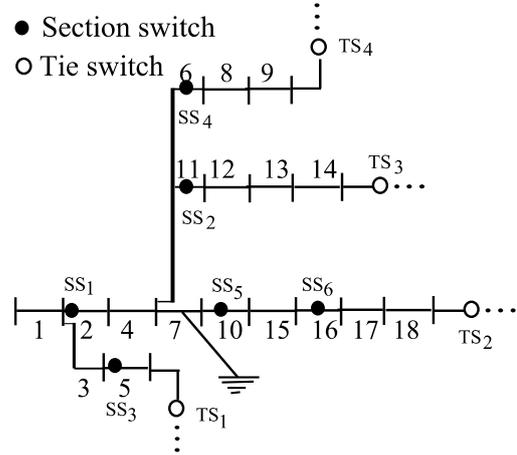
Figure 2: Feeder with switches installed considering a fault in line section 7.
