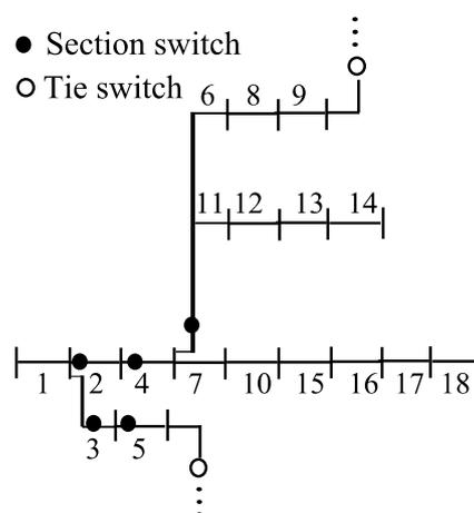
Figure 1: Example of tie switches allocated downstream of section switches.
