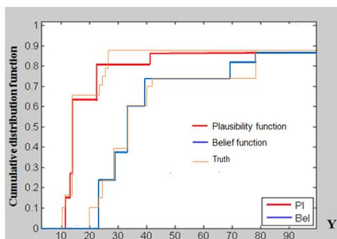
Figure 6: Belief and plausibility functions of the combined parameter and structural model imperfections for LCCs.
