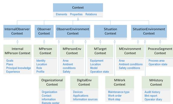
Figure 2: A class diagram presenting MaintenanceContext classes (two lower rows) in SituationAssessment context hierarchy (two upper rows). Some examples of the possible Elements of the Context classes are listed as class members.
