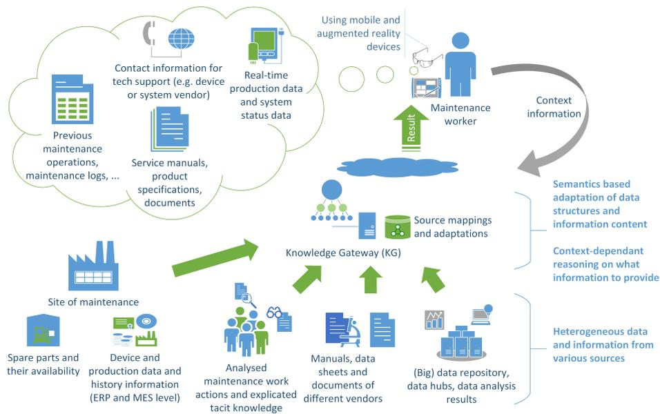
Figure 1: The maintenance knowledge management concept is based on a knowledge gateway (KG) that combines information from various sources in a meaningful way based on semantic descriptions and reasoning of the context.
