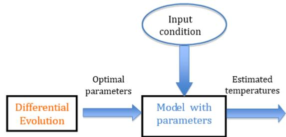
Figure 1: DE, parameterized model, and temperature estimation.
