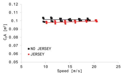
Figure 6: Experimental results from the mannequin test with and without jersey.
