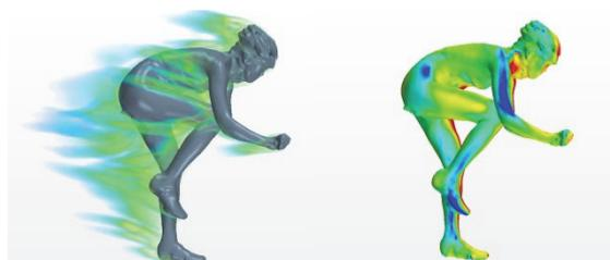
Figure 12: Vorticity field around the full model. And pressure contour plots on the model.
