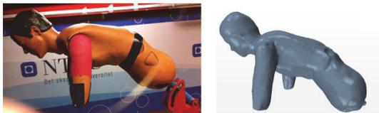
Figure 3: Mannequin model in the wind tunnel (left) and 3D laser scanned model (right).
