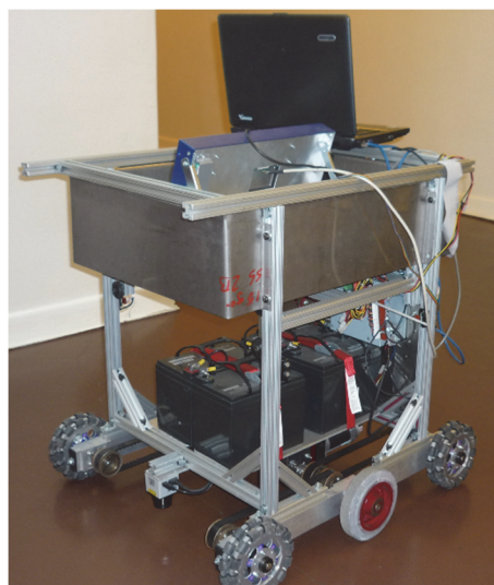
Figure 1: Robot with a laser scanner (between the front wheels).
