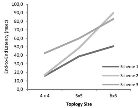
Figure 14: End-to-end latency measured for low priority data in schemes 1, 2 and 3.
