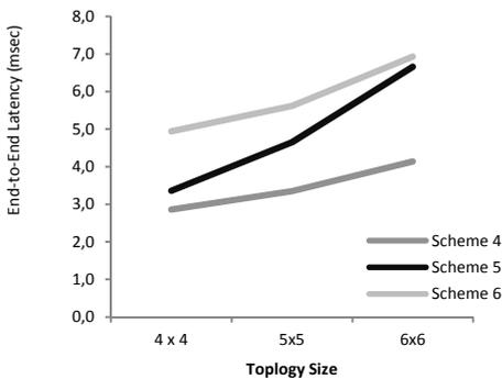
Figure 13: End-to-end latency measured for medium priority data in schemes 4, 5 and 6.
