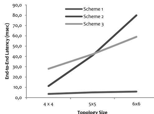
Figure 10: End-to-end latency measured for high priority data in schemes 1, 2 and 3.
