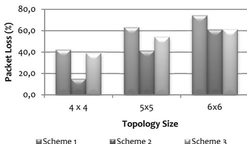
Figure 6: Packet loss for medium priority data for schemes 1, 2 and 3.
