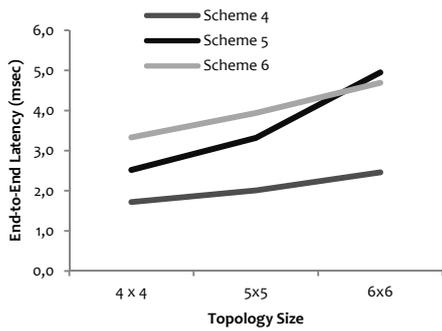
Figure 11: End-to-end latency measured for high priority data in schemes 4, 5 and 6.
