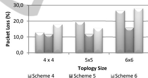
Figure 9: Packet loss for low priority data for schemes 4, 5 and 6.
