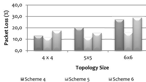
Figure 7: Packet loss for medium priority data for schemes 4, 5 and 6.
