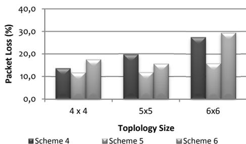
Figure 5: Packet loss for high priority data for schemes 4, 5 and 6.
