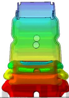
Figure 12: Strain distribution in the crash box before and after deformation (Ambrozinski et al., 2015).
