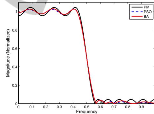
Figure 7: Normalized plot for the low pass FIR filter of order 24.
