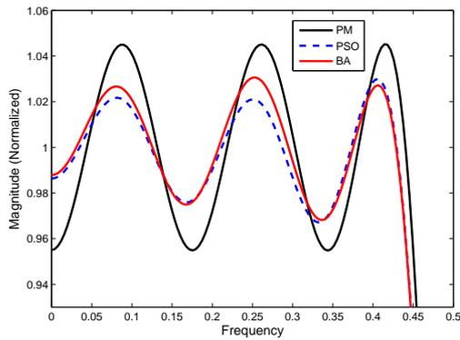
Figure 8: Normalized pass band ripple plot for the low pass FIR filter of order 24.
