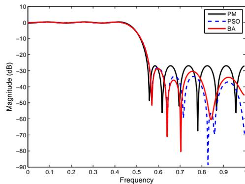
Figure 10: Magnitude (dB) plot for the low pass FIR filter of order 24.
