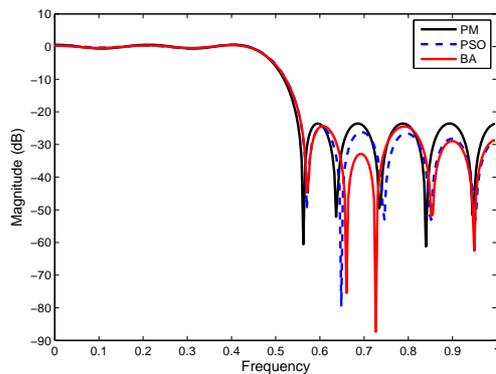
Figure 5: Magnitude (dB) plot for the low pass FIR filter of order 20.
