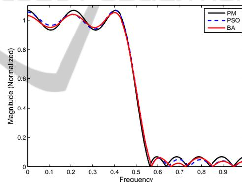
Figure 2: Normalized plot for the low pass FIR filter of order 20.
