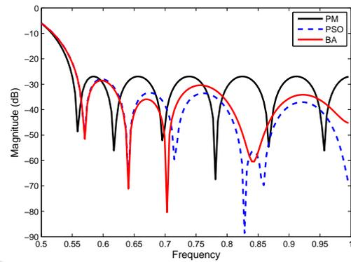
Figure 11: Magnitude (dB) plot for the stop band of low pass FIR filter of order 24.
