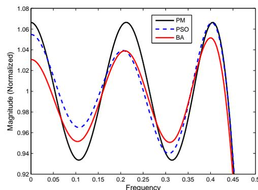
Figure 3: Normalized pass band ripple plot for the low pass FIR filter of order 20.
