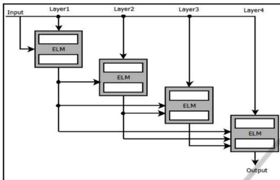
Figure 8: Schematic of full cascade ELM.
