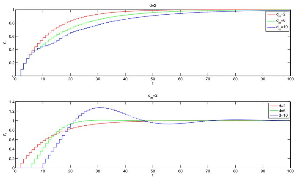
Figure 6: Step responses for nmph system with controller (35).
