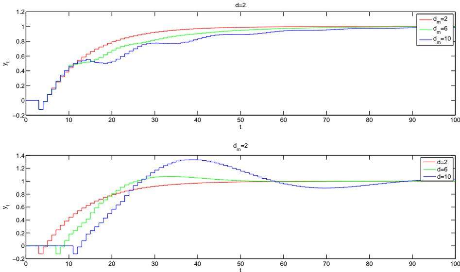
Figure 4: Step responses for nmph system with controller (27).
