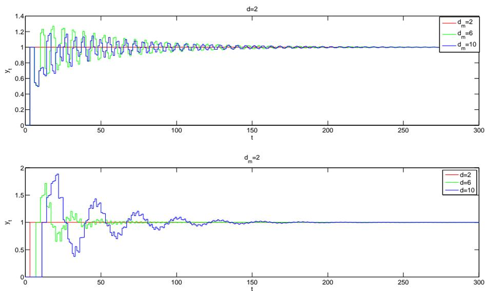
Figure 2: Step responses for stable system with controller (31).
