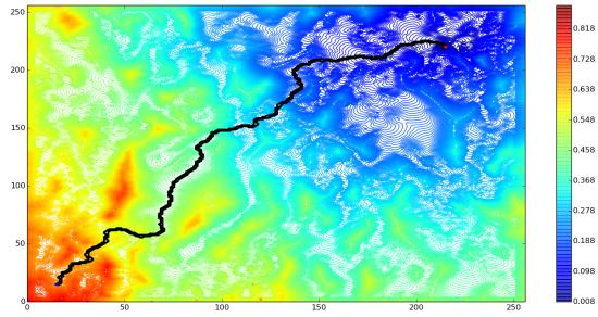
Figure 10: *Scenario 1* - Path planning over the representation of the isochrone lines of the processed surface represented in Fig. 4.
