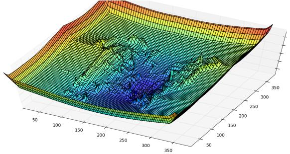
Figure 9: *Scenario 3* - Energy potential representation of the processed Fig. 8 with the goal set at (184,203) which is the top of a simulated flight of stairs.
