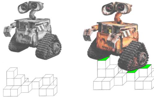
Figure 1: Conceptualization of the problem of determining the resting pose of the UGV on the terrain surface by means of virtually dropping it from a height.
