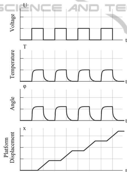
Figure 10: Motion cyclogram of the microrobot leg.
