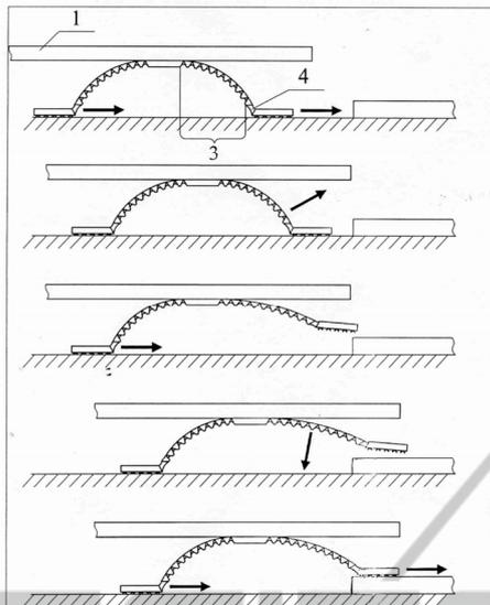
Figure 9: Mode of motion of the mobile microrobot along a stepped surface.
