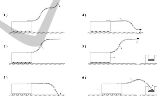
Figure 12: Inspector microrobot taking ground samples.
