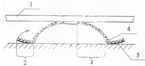
Figure 4: Design of a microrobot leg (version one).
