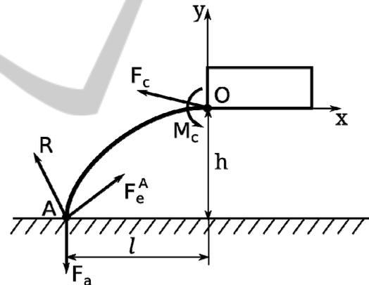
Figure 3: Forces and torques acting on the robot's leg.
