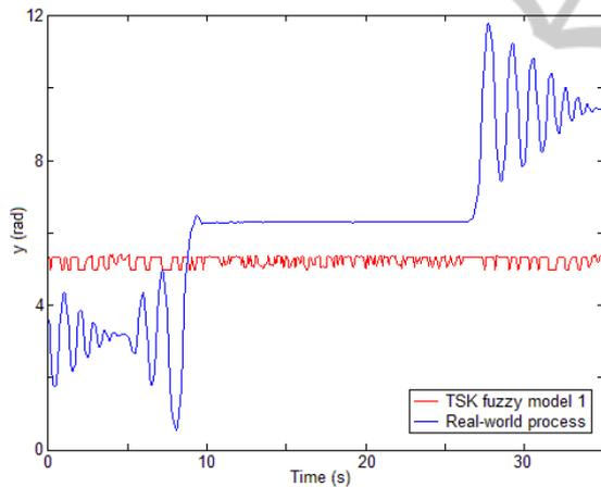
Figure 2: Pendulum angle versus time of TSK fuzzy model 1 and of real-world process for validation data.
