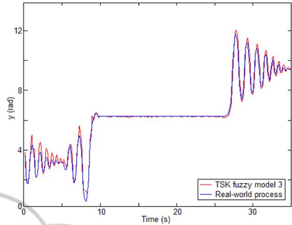
Figure 4: Pendulum angle versus time of TSK fuzzy model 3 and of real-world process for validation data.
