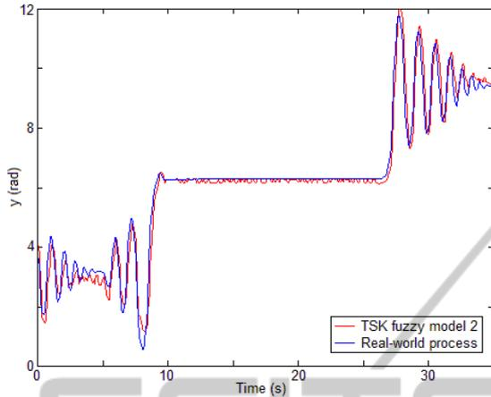
Figure 3: Pendulum angle versus time of TSK fuzzy model 2 and of real-world process for validation data.
