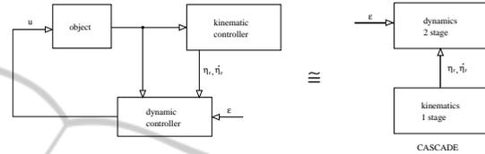
Figure 2: Structure of the proposed control algorithm: cascade with two stages.
