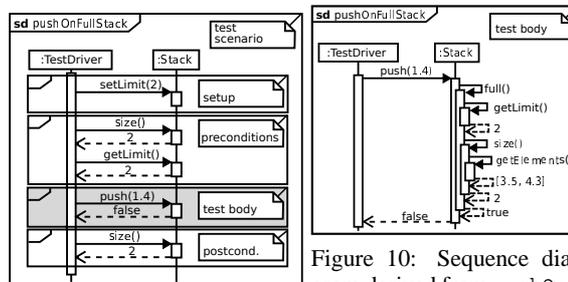
Figure 9: Sequence diagram derived from pushOnFullStack zooming in on derived from pushOnfull-test body and representing Stack highlighting calls both, calls running from running from STF to SUT. STF to SUT and calls internal to the SUT.
