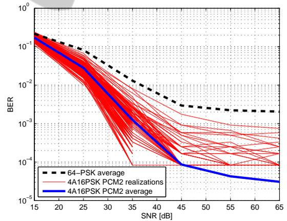
Figure 4: BER versus SNR results for “Flying Platform” scenario ( $f_0 = 4 \text{ GHz}$ ).
