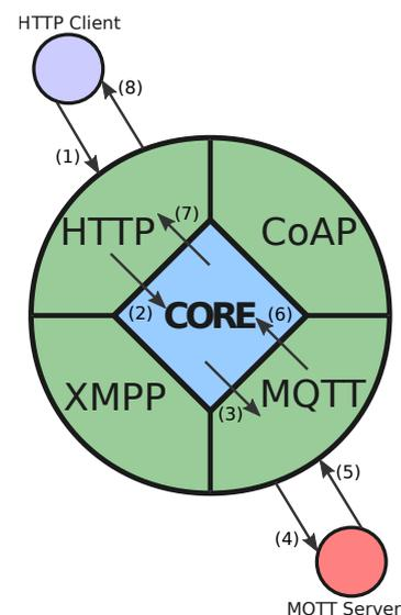
Figure 3: The flow throughout the gateway of a HTTP-MQTT request.
