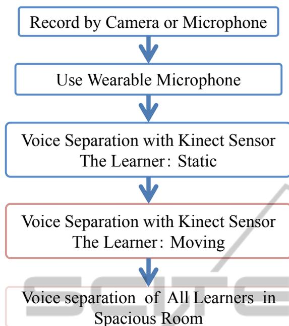
Figure 3: Flowchart of the developed technology.
