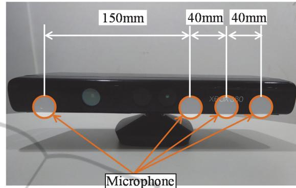
Figure 5: Photograph of the Kinect sensor.
