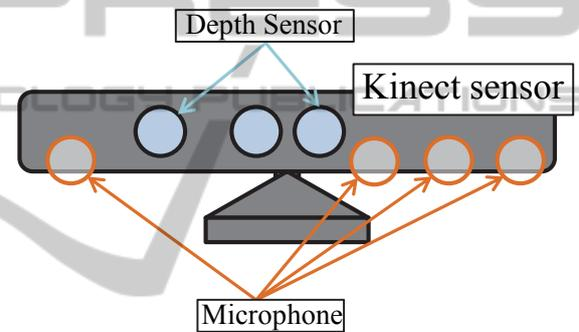
Figure 6: Kinect sensor.
