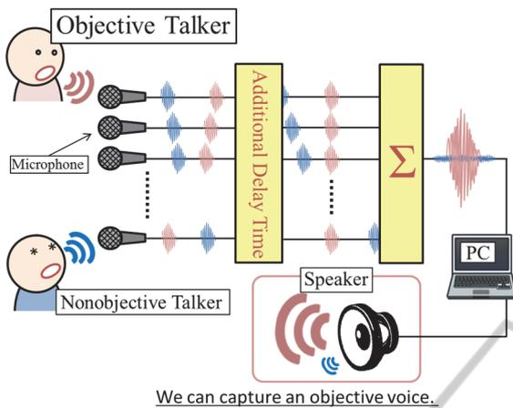
Figure 4: Schematic of the DSBF method.
