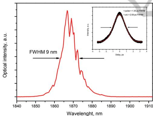
Figure 6: Spectrum and autocorrelation for the mode-locked Tm-doped laser operating in normal dispersion regime.
