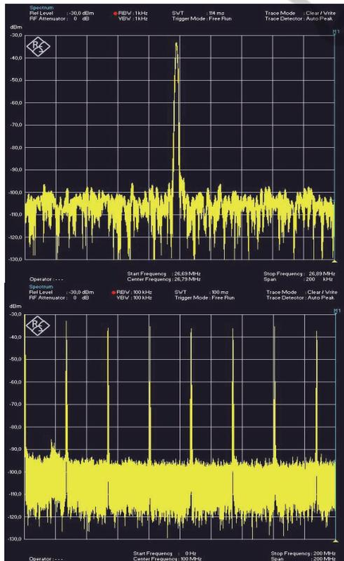
Figure 3: Measured RF spectrum of mode-locked output: with a 200 kHz frequency span and 1 kHz resolution bandwidth (upper); with a 200 MHz frequency span and 100 kHz resolution bandwidth, showing a broad spectrum of harmonics (lower).
