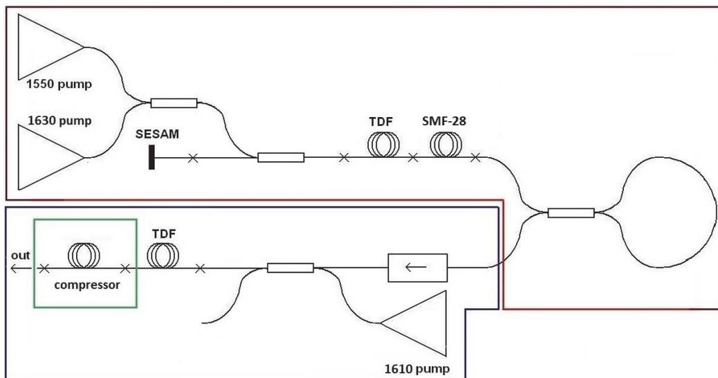
Figure 1: The schematic of the TDF laser (red frame) and amplifier (blue frame).
