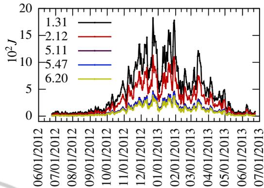
Figure 2: Maximum multi-commodity flow solutions (daily duty cycling, second floor sink, various  $q/p$ ).
