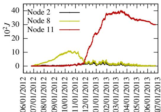
Figure 17: Residual energy at nodes 2 and 8 (both adjacent to the sink) and node 11 (3rd floor), with sink at the fourth floor.
