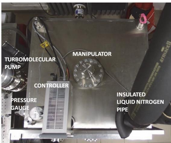
Figure 1: Top view of the vacuum chamber.
