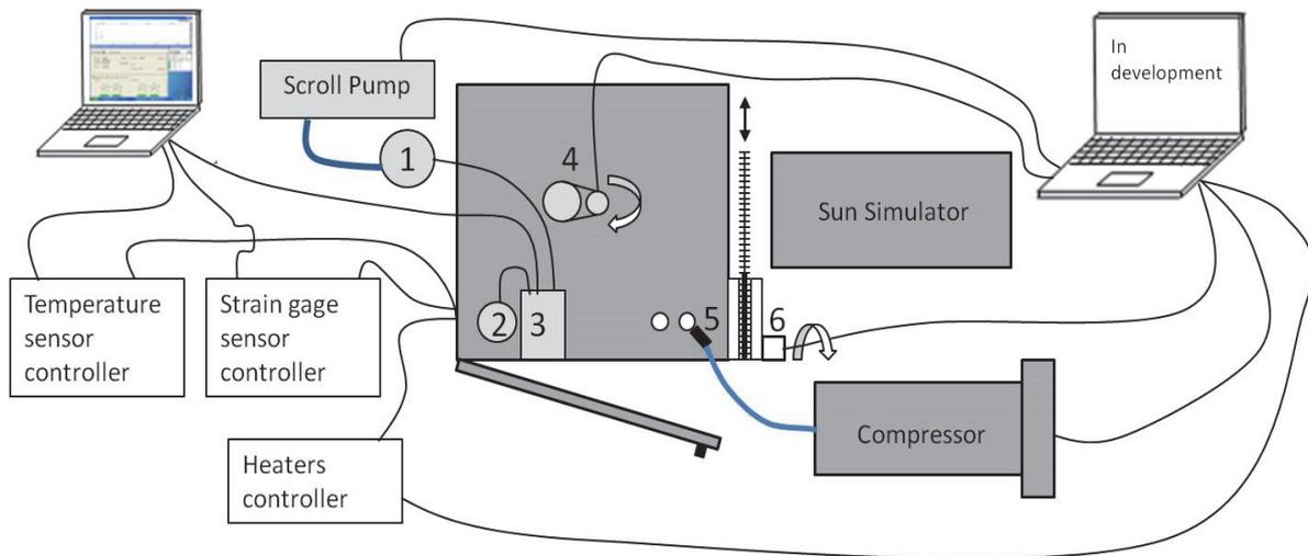
Figure 5: Full automation of thermo-vacuum facility. Left part is operational, right part is under development. 1- turbomolecular pump, 2- pressure gauge, 3- turbomolecular pump and pressure gauge controller, 4- manipulator and stepper motor, 5- cryogenic valve with pneumatic actuation (see Figure 6), 6- stepper motor for sun simulator diaphragm.
