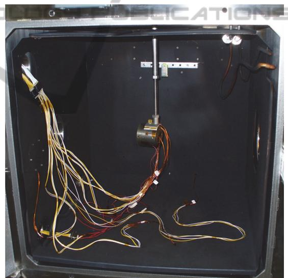
Figure 2: Front view of the open vacuum chamber. The specimen under test, is mounted on the axis of the manipulator. The cables connect the temperature sensors and the resistive heaters to the external acquisition system. The black walls are the liquid nitrogen cooled shrouds. The sun simulator is outside of the right window.
