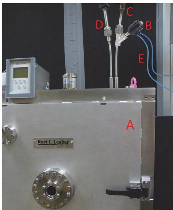
Figure 6: Pneumatic actuated valve. The vacuum chamber (A) is equipped with liquid nitrogen cooled shrouds. The valve (B) will be fitted to the input nitrogen pipe (C). The nitrogen leaves the cooling circuit from the output pipe (D). The valve is operated by controlling the flux of pressurized air, in the blue pipes (E).
