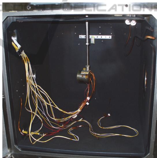
Figure 2: Front view of the open vacuum chamber. The specimen under test, is mounted on the axis of the manipulator. The cables connect the temperature sensors and the resistive heaters to the external acquisition system. The black walls are the liquid nitrogen cooled shrouds. The sun simulator is outside of the right window.
