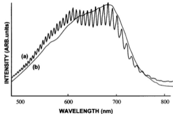
Figure 4: The plot taken from Sharma, et al 1998 is showing the spectrum of (a) the SMF with coating and (b) without coating.
