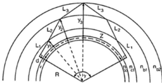
Figure 2: Schematic of the WGM interference model from Morgan et al 1990. The dashed line is the fundamental mode traveling along the fibre core, the continues line is radiation traveling from the core to the cladding until strike the second coating-air interface, and then going back to the cladding.
