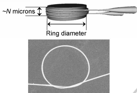
Figure 8: On top, example of a micro coil resonator taken from Sumetzki, 2008. On bottom, picture of a knot resonator made using an optical fibre microwire (Brambilla, et al 2009).
