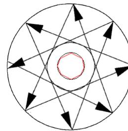
Figure 6: Schematics of helicoidal (skew) modes bouncing along a fibre coating. Figure modified from Su, et al 1992.
