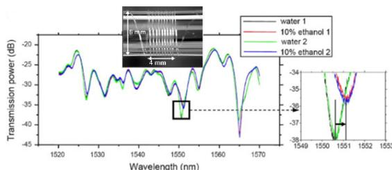
Figure 5: Variations of transmission of a micro-fibre coil resonator immersed in water and ethanol. The inset is the picture of the tested micro-fibre coil. On the right hand of the picture is a close-up showing the shift of the oscillations due to refractive index change of the measured sample. Picture adapted from Sumetsky, et al 2010a.
