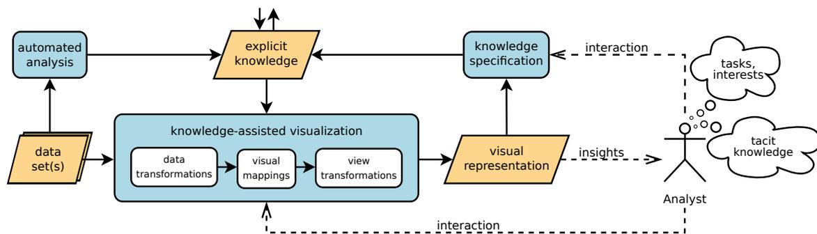
Figure 1: This image shows the integration of explicit knowledge for knowledge-assisted visualizations in the visual analytics process.
