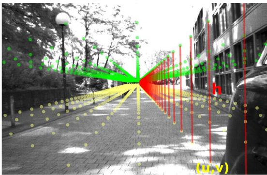
Figure 4: Calculate the distance  $h$  between each point pair and store it. Location  $(u, v)$  is the coordinates of the corresponding ground point.
