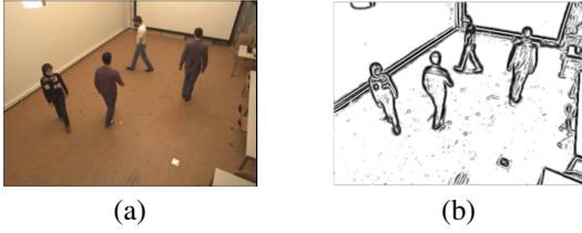
Figure 3: (a) Input image. (b) Gradient confidence levels, where darker means more likely. Note that all clear edges in the image are represented by similarly strong gradient confidences.
