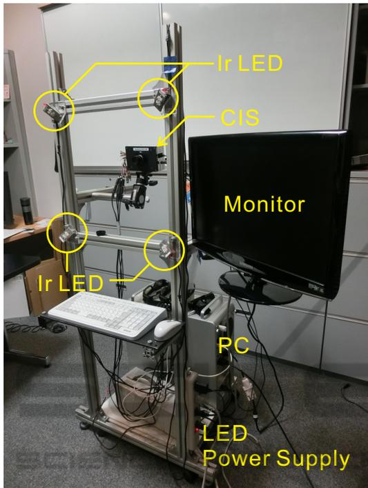
Figure 4: Photograph of real time surface orientation imaging system.
