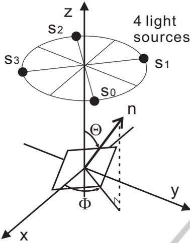
Figure 3: Geometry of quadrature phase light sources and surface normal.
