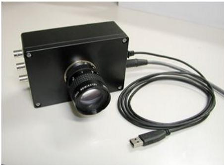
Figure 1: Photograph of Correlation Image Sensor(CIS).
