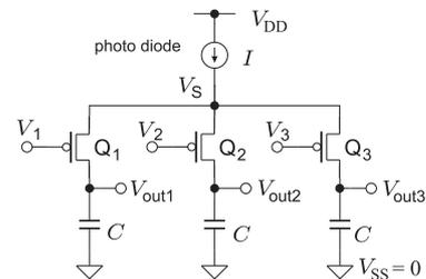
Figure 2: Pixel structure of the correlation image sensor.
