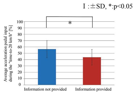
Figure 11: Average Acceleration Pedal Input During the "Time-to-20 km/h".
