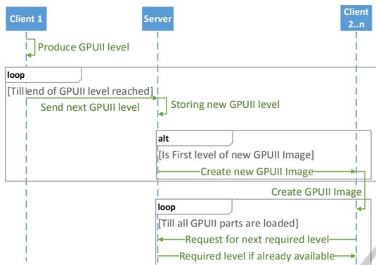
Figure 2: Sequence diagram for upload and distribution of a newly captured and positioned photo using GPU image levels.
