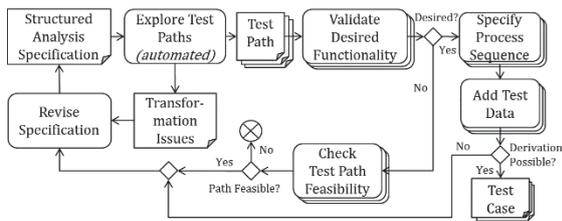
Figure 2: Review Process Supported by Test Paths.
