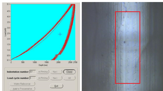
Figure 5: On the left, snapshot of the 17 best loading curves. On the right, a picture of the area selected after nanoindentation.
