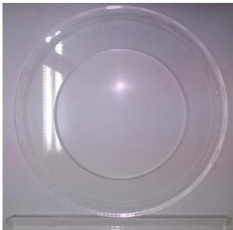
Figure 5: The fabricated PMMA waveguide and PMMA ring resonator.
