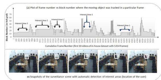
Figure 5: (a) Evidence of the presence of interest point in temporal domain on a set of trajectories selected from the in-house dataset. (b) A few snapshots of the surveillance scene where the interest point was automatically marked when a person reached the location of interest.
