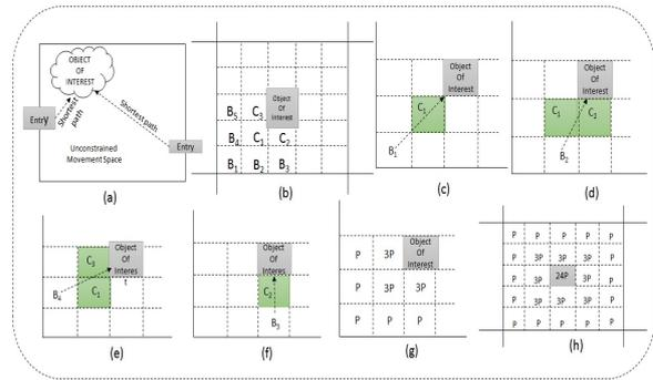
Figure 1: (a) A typical representation of the surveillance environment with one object of interest. (b) Rectangular sub-division of the surveillance environment assuming the object of interest is located at the center. (c-f) Typical motion pattern followed by a target while approaching the static object of interest. (g-h) Estimation of importance of a block as a function of the motion dynamics.
