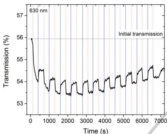
Figure 3: Observation of reversible transient PD in  $(\text{GeSe}_2)_{90}(\text{Sb}_2\text{Se}_3)_{10}$  PLD thin films irradiated at 593 nm during 2 hrs. Dotted red line corresponds to pump beam turn on and blue line to pump beam turn off.
