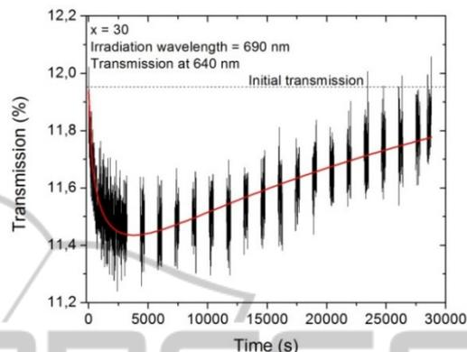
Figure 2: Evolution of transmission at  $640 \text{ nm}$  for an as-deposited film ( $x=30$ ) under  $690 \text{ nm}$  irradiation light (8 hours exposure).
