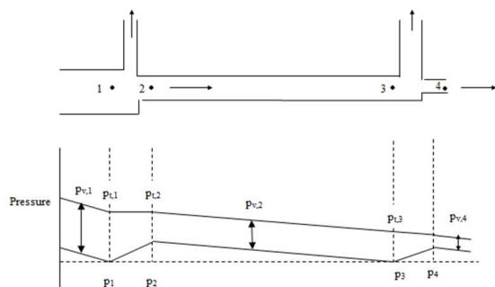
Figure 1: Schematic of pressure distribution for static regain design, where  $p_t$  = total pressure,  $p$  = static pressure and  $p_v$  = velocity or dynamic pressure (Mitchel and Braun, 2012).
