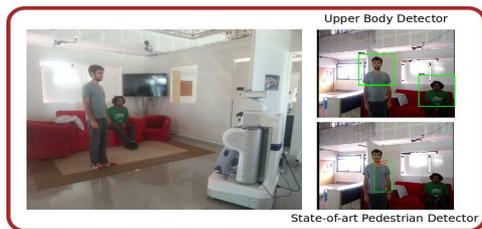
Figure 1: Output of our proposed detector (top right) and state-of-art pedestrian detector (Dollár et al., 2014), bottom right, in an HRI context.
