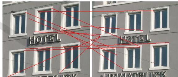
Figure 1: Example from the Zurich Building Image Database of repetitive patterns leading in "good-false" matches with the sift descriptor.
