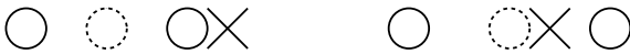
Figure 6: Circles: two inaccurate detections, one from the current frame and one shifted from the last frame. Dotted circle: Average position of the two circles. Cross: ground truth. Only in the right example the dotted circle is closer to the ground truth than the average distance of the two normal circles to the ground truth. As the position variations of the eye detector is mostly like on the left (one sided error) there is no big benefit for our information fusion approach in average pixel location error. However, the dotted circle is less noisy in position than the original circles which supports prediction (see text).
